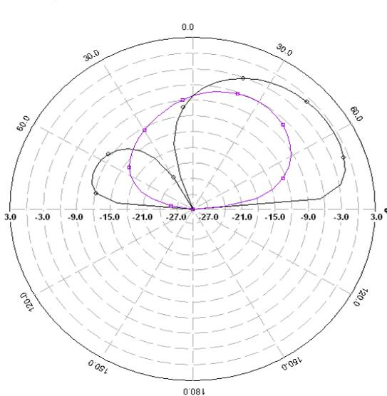
**Fig. 7(d)** Radiation Pattern at 6.3 GHz
