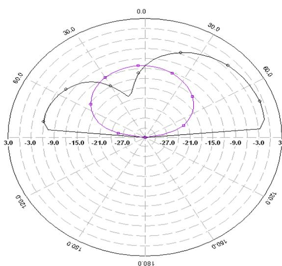
**Fig. 7 (a)** Radiation Pattern at 2.63 GHz
