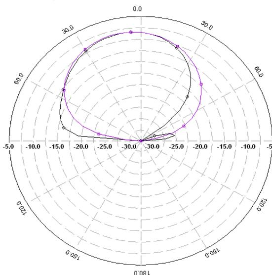
**Fig. 7(c)** Radiation Pattern at 4.79 GHz
