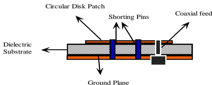
Figure 2: Side view of proposed antenna
