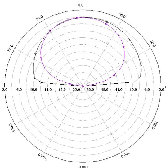
**Fig. 7 (b)** Radiation Pattern at 3.12 GHz
